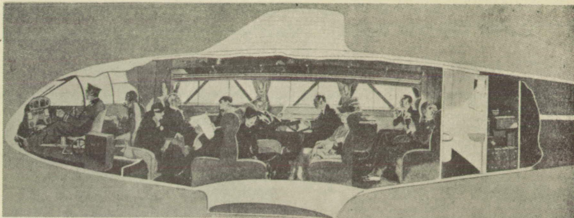
Figure 2.-An artist's impression of the inside of the D.H. 86 "Express Air Liner" showing the seating arrangement for ten passengers. It can be seen how light and comfortable the cabin is.
