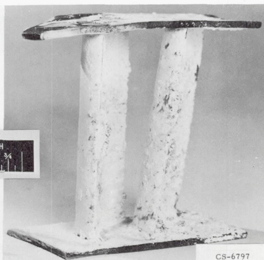
Figure 8. - Boron oxide deposits from diborane on turbine stator blades.
