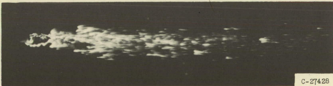
(c) 30-percent slurry of magnesium containing gelling agent; apparent viscosity, 800 to 1600 centipoises.
