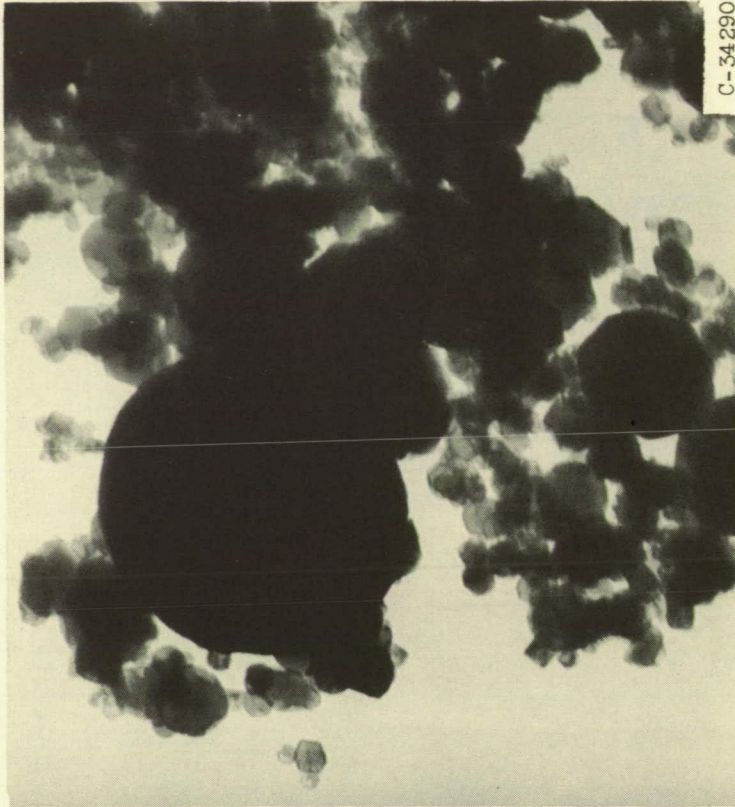
Figure 3. - Electron micrographs of two representative fields of magnesium particles magnified 25,000 times (ref. 19).
