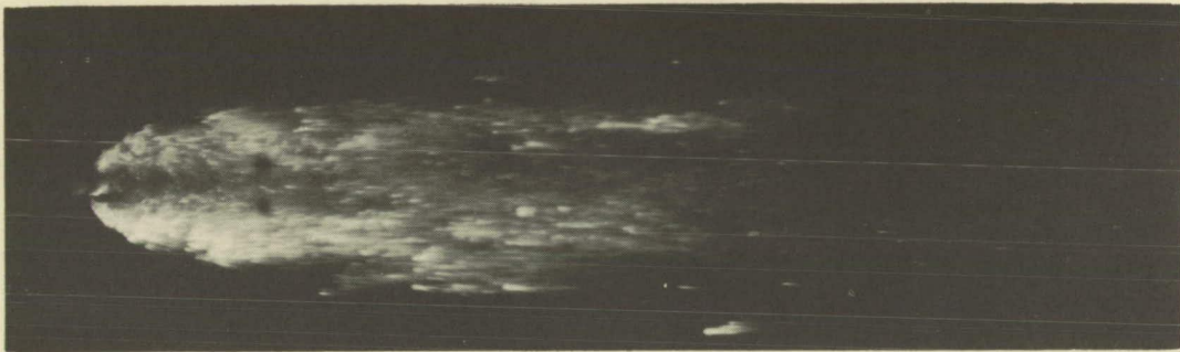
(b) 30-percent slurry of magnesium containing gelling agent; apparent viscosity, 300 to 400 centipoises.
