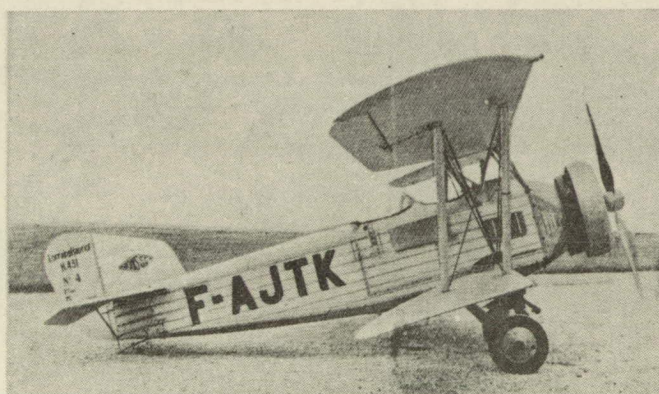
Fig. 3 Side view of the Lorraine-Hanriot H-431 showing the annular cowling of the "Mizar" type.
