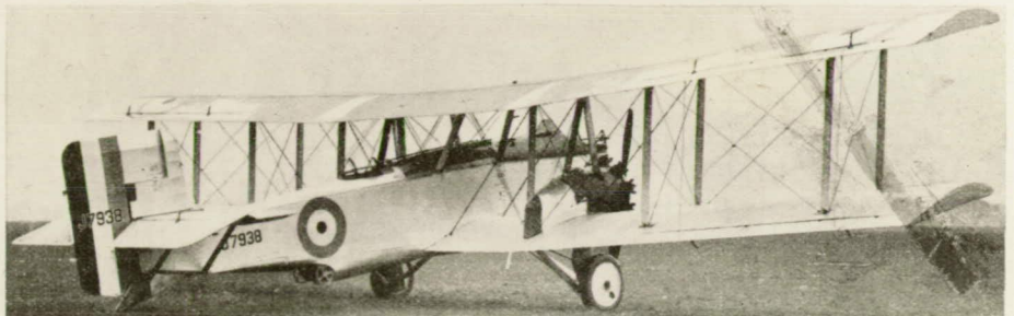
Fig. 3 Three-quarter rear view of the "Sidestrand I". The careful streamlining of the engine nacelle is apparent.
