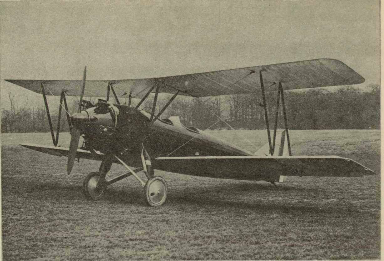
Fig. 3 Three-quarter front view of the "Avro Trainer" airplane. The fabric fairings are made as detachable units to facilitate inspection of the fuselage structure. "Flight" photographs reproduced by permission
