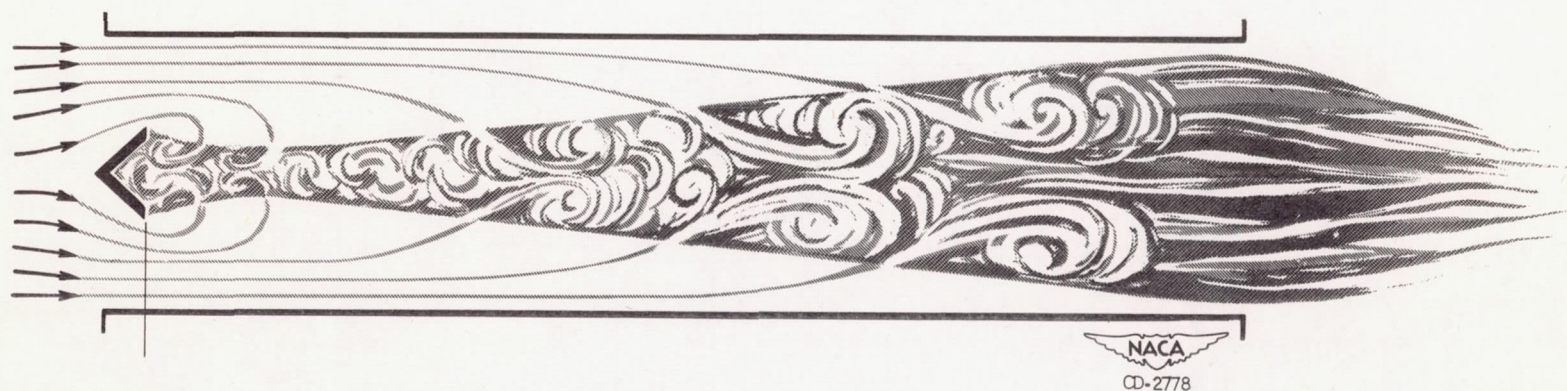
Figure 10. - Schematic illustration of instantaneous cross section of flame in 5-inch ram-jet-type combustor.
