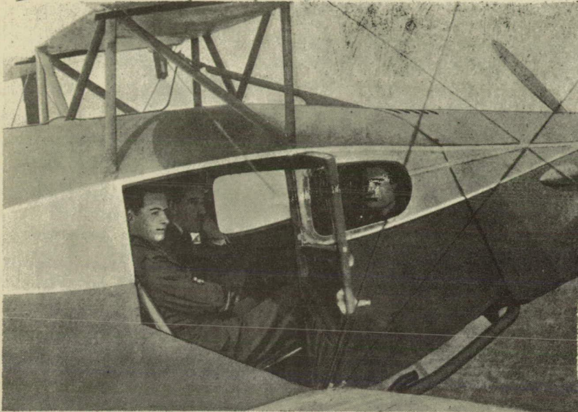
Fig.10 View of Fox Moth showing third passenger seated facing aft. From "Aeroplane"
