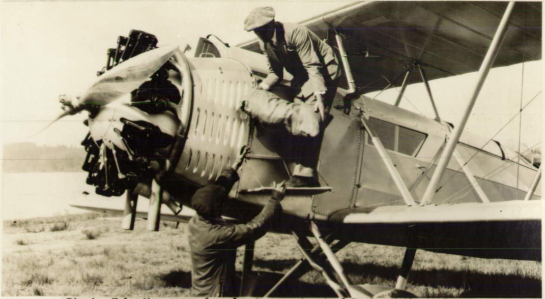
Fig.4 Unloading cargo from front compartment of Boeing Mail airplane
