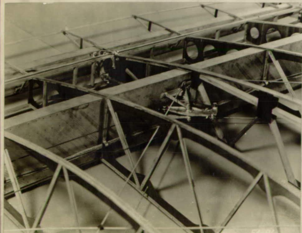
Fig. 6 Alleron controls are entirely inside of the wings. Note the bell-crank mechanism that makes it possible to run wires straight and thus eliminate all pulleys. Control cables last indefinitely, eliminating the necessity of replacing them from time to time.
