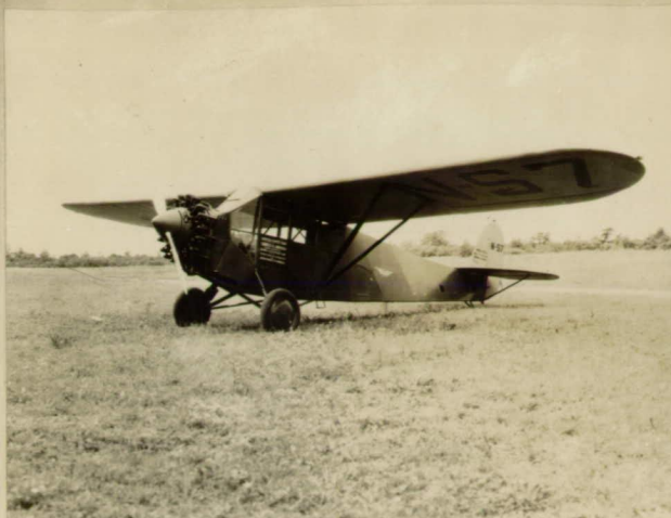
Fig. 2 The Fairchild "All-purpose" cabin monoplane. The cabin provides seats for five, the pilot being located at the extreme front with the passengers seated in pairs back of him.
