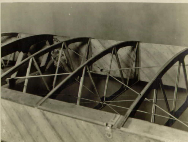
Fig. 7 The rugged wing construction is built to withstand hard usage. With its substantially constructed spars, well proportioned ribs and carefully designed fittings this claim is reasonably substantiated.
