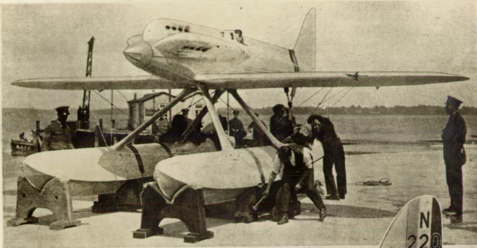
Fig. 1 Views of the Supermarine S.5 seaplane, giving an excellent idea of the clean lines. Note particularly how neatly "the Napier" "Lion" racing engine is faired into the fuselage.
