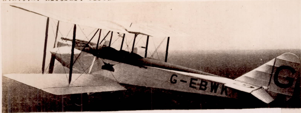
Figs. 2 & 3 Views of the Avro "Avian III" air- plane. Note the neat cowl- ing at the nose.
