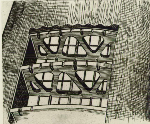
Fig.5 Interior of fuselage looking aft. The open passage can be used during flight to inspect the steering controls and the tail-skid shock absorbers.
