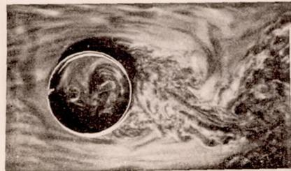
Figs.10-13 Flow around a cylinder in various phases of development.
