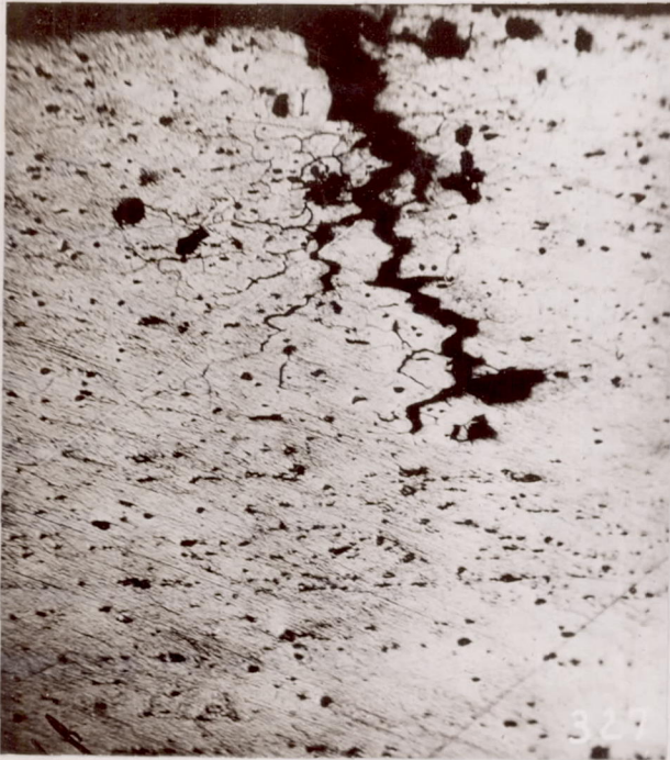
Fig.1 Severe intercrystalline corrosion magnified to 100X.
