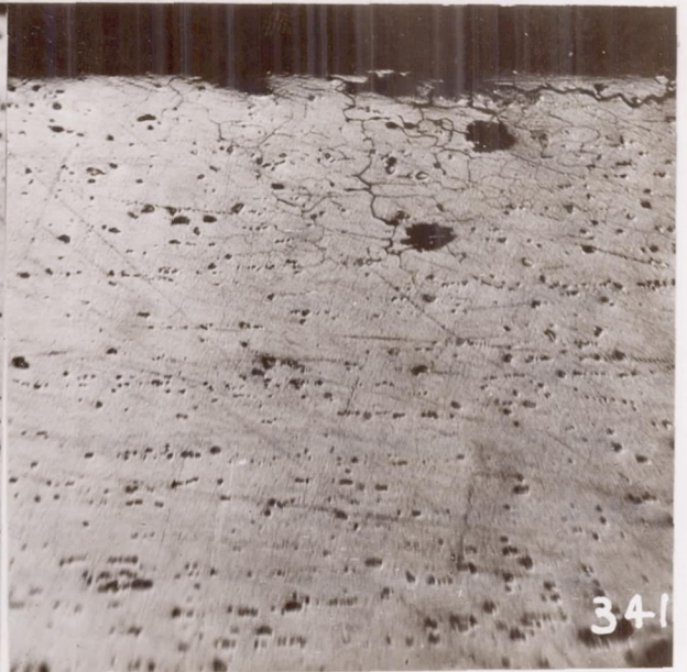
Fig.2 Intercrystalline corrosion in duralumin as brought out by etching.
