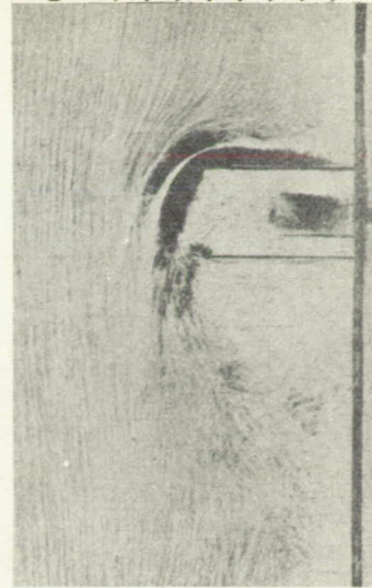
Fig. 10 Flow about a pair of screens.
