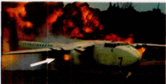
(b) Ignition right nacelle, test 7; 3.5 seconds after initial impact. Airplane speed, 50 feet per second.
