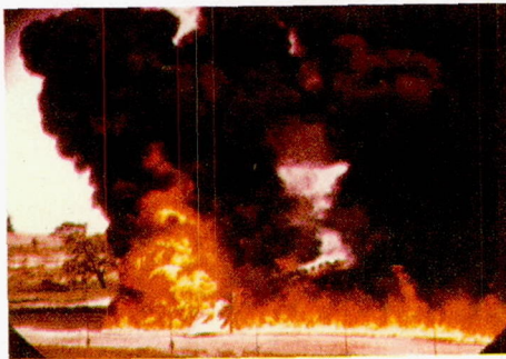
(c) Fire from fuel evaporating from wetted surface of airplane and ground; 10.0 seconds after ignition.
