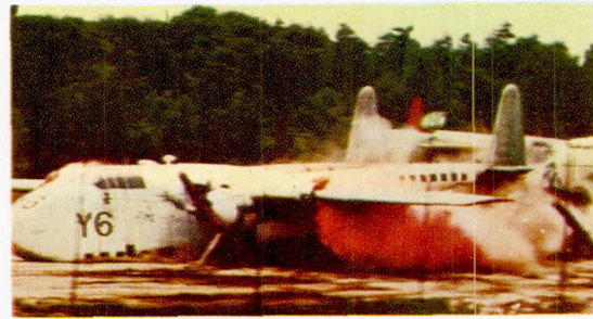
(b) Side view; 0.37 second after impact with first pole barrier. Airplane speed, 125 feet per second.
