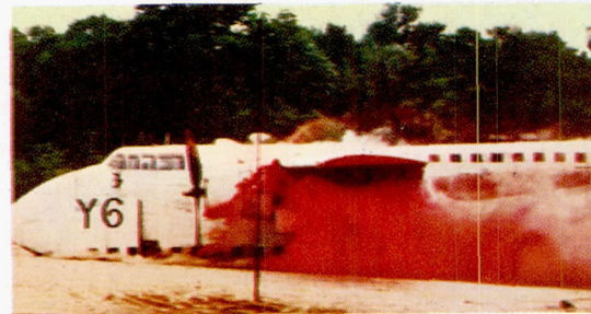
(f) Side view; 3.4 seconds after impact with first pole barrier. Airplane speed, 20 feet per second.
