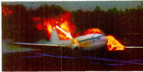
(a) Fire 2.8 seconds after initial impact. Airplane speed, 42 feet per second.
