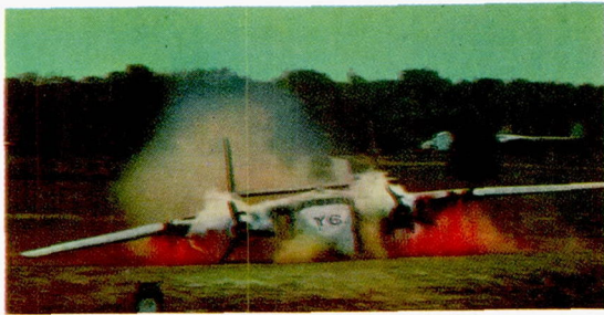
(g) Front view; 4.4 seconds after impact with first pole barrier. Airplane speed, 8 feet per second.
