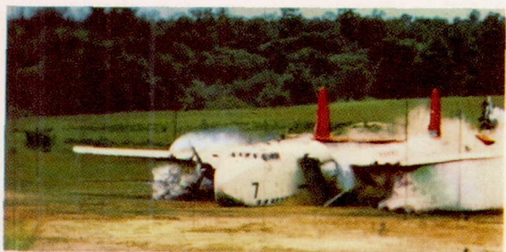
(a) Engine cowl disruption at barrier; 1.0 second after initial impact. Airplane speed, 130 feet per second.
