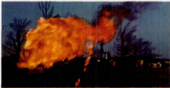
(c) Propagation of flame upwind in mist of aviation gasoline.
