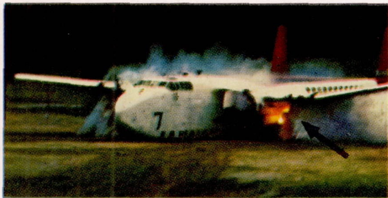
(a) Ignition left nacelle, test 7; 2.0 seconds after initial impact. Airplane speed, approximately 98 feet per second.
