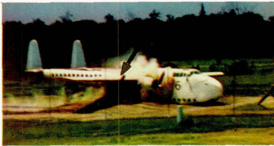
(a) Impact of poles with landing lights; 0.25 second after initial impact. Airplane speed, 143 feet per second.
