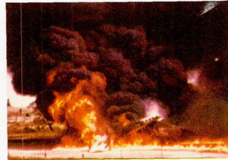
(d) Fire produced by fuel that soaked into ground vaporizing and burning in column continuous with burning fuel from tanks; 19.0 seconds after ignition.
