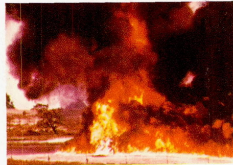
(b) Fuel mist fire with rising column of smoke and burning core of fuel mist; 5.3 seconds after ignition.
