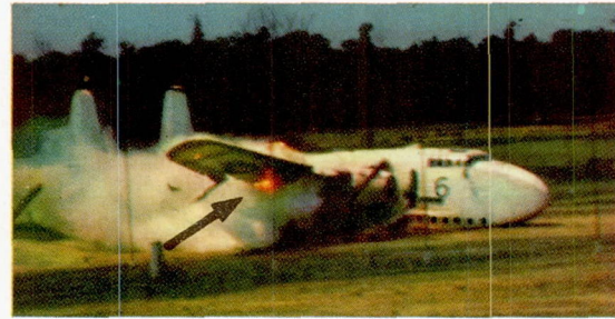
(b) Ignition on right side of airplane; 0.60 second after initial impact. Airplane speed, 135 feet per second.
