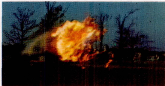
(b) Propagation of flame downwind in mist of aviation gasoline.
