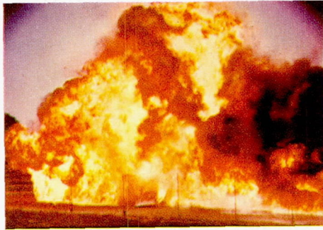
(a) Fuel mist fire at its maximum; 3.0 seconds after ignition.
