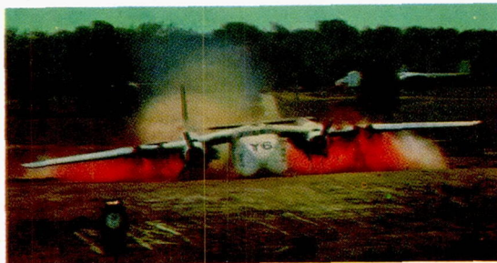
(e) Front view; 3.0 seconds after impact with first pole barrier. Airplane speed, 30 feet per second.
