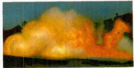
(d) Spread of fire 3.9 seconds after initial impact. Airplane speed, 0.
