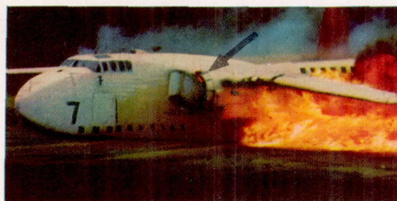
(b) Induction-system fuel ignition 3.5 seconds after initial impact. Airplane speed, 50 feet per second.
