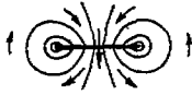
FIG. 33.—Acceleration diagram around an infinitely long flat plate accelerated at right angle to its surface.
