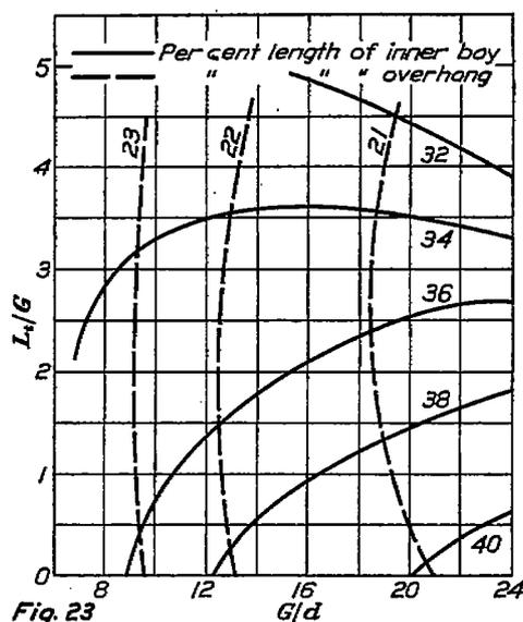
of only 1 per cent, or an increase of one-half of 1 per cent, in overhang has as much effect. When  $G/d$  is 8, the triangular figures of equal moment are more nearly equilateral, and the locations of inner and outer struts are of more nearly equal importance.
