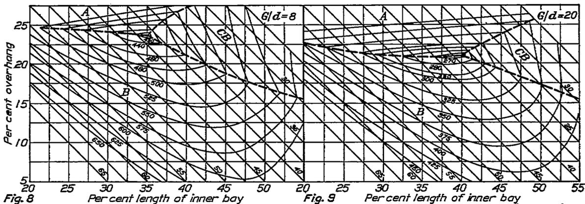
at two values of  $G/d$  are given in Figures 8 and 9, and those for the lower spar for a single value in Figure 10. The diagonals sloping downward and to the right give the length of the outer bay.
