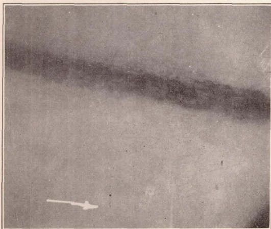
Injection pressure 1,500 lbs./sq. in. 0.008 in. (0.02 mm) orifice diameter 1\frac{5}{16} in. (2.4 cm) from orifice
