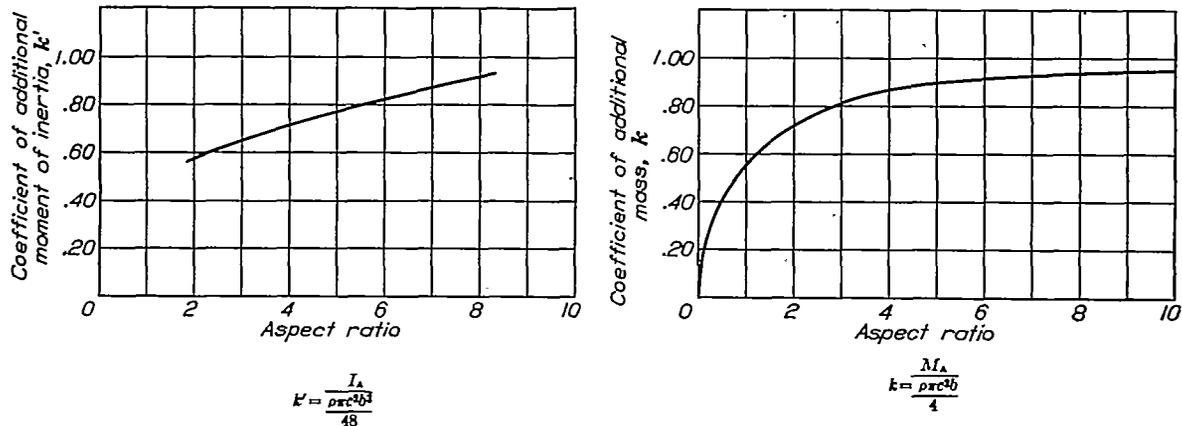
FIGURE 3.—Coefficients of additional mass and additional moments of inertia for flat plates.
