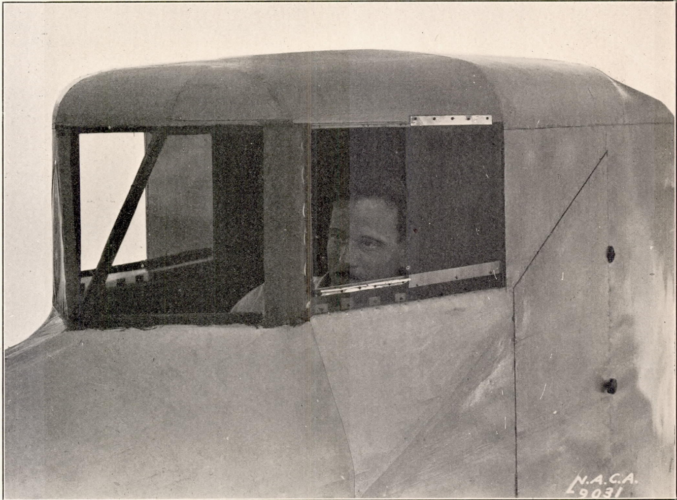
FIGURE 22.—Windshield 6B showing position of pilot's head required to obtain forward vision.
