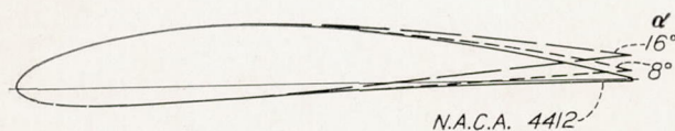
FIGURE 12.—Change in profile shape associated with the modified theoretical calculation of pressure.
