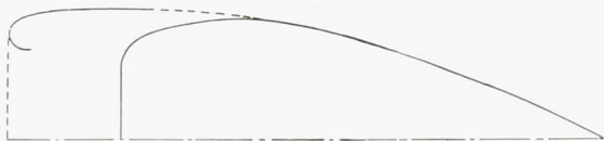
FIGURE 1.—Basic cowling shape for determining minimum drag.
