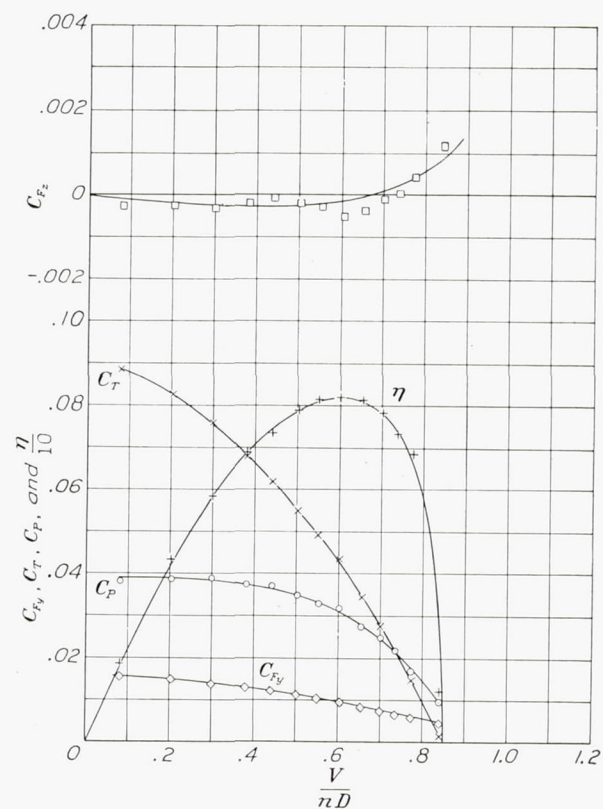
FIGURE 7.—Characteristics of a propeller set 16.6° at 0.75R; 10° yaw.
