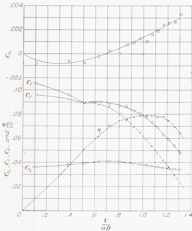
FIGURE 20.—Characteristics of a propeller set 28.6° at 0.75R; 20° yaw.
