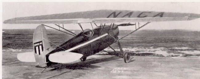
FIGURE 2.—Fairchild 22 airplane used for tests of conventional ailerons on a tapered wing.
