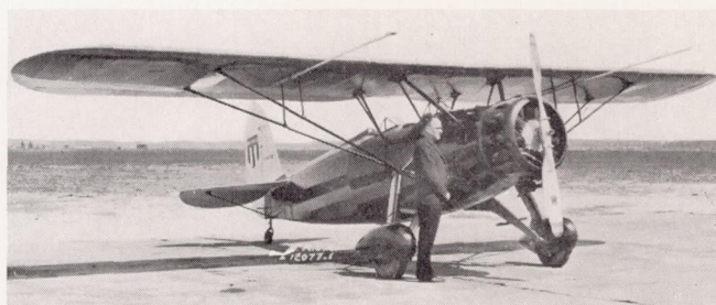
FIGURE 1.—Fairchild 22 airplane used for tests of conventional ailerons on a rectangular wing.
