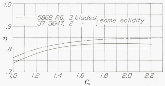
FIGURE 40.—Efficiency-curve envelopes for two propellers having the same solidity but a different number of blades.
