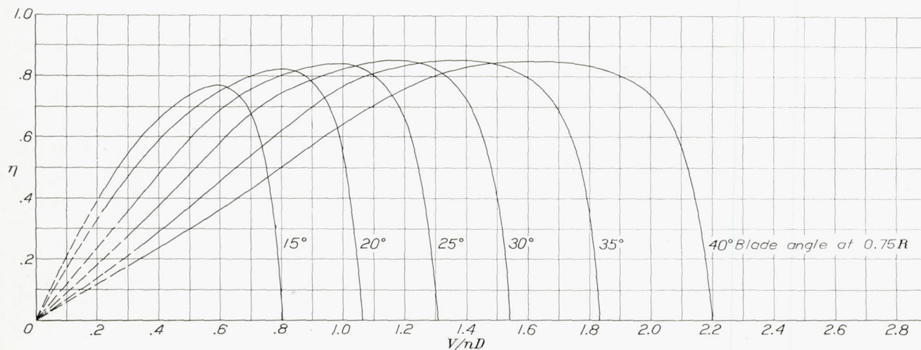
FIGURE 19.—Efficiency curves for propeller 6129, 3 blades, radial engine nacelle.
