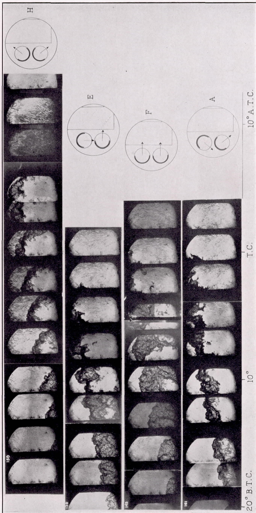
FIGURE 6.—Effect of gas movement on combustion. Engine speed, 500 r. p. m.; one spark plug.
