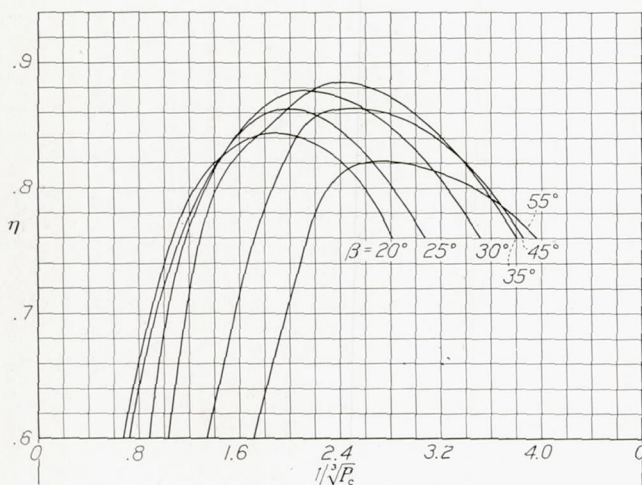
FIGURE 30.—Curves of propulsive efficiency against 1/\sqrt{P_c} for propeller C on nose 5.
