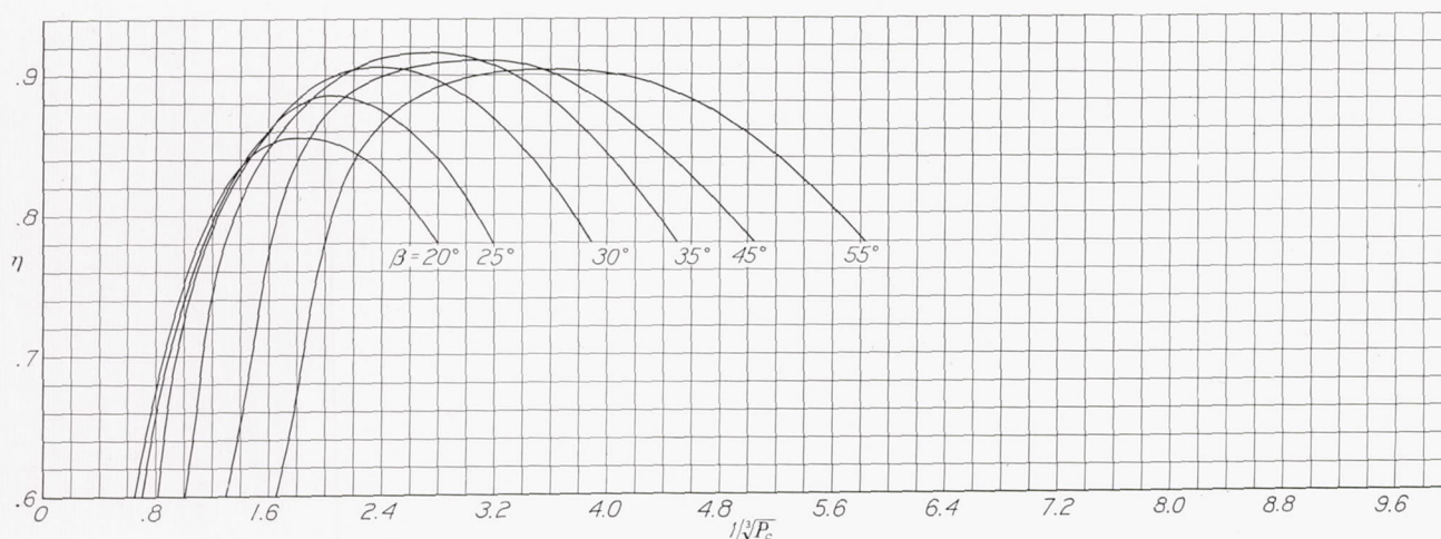
FIGURE 25.—Curves of propulsive efficiency against 1/\sqrt{P_c} for propeller F on nose 3 with spinner 1.
