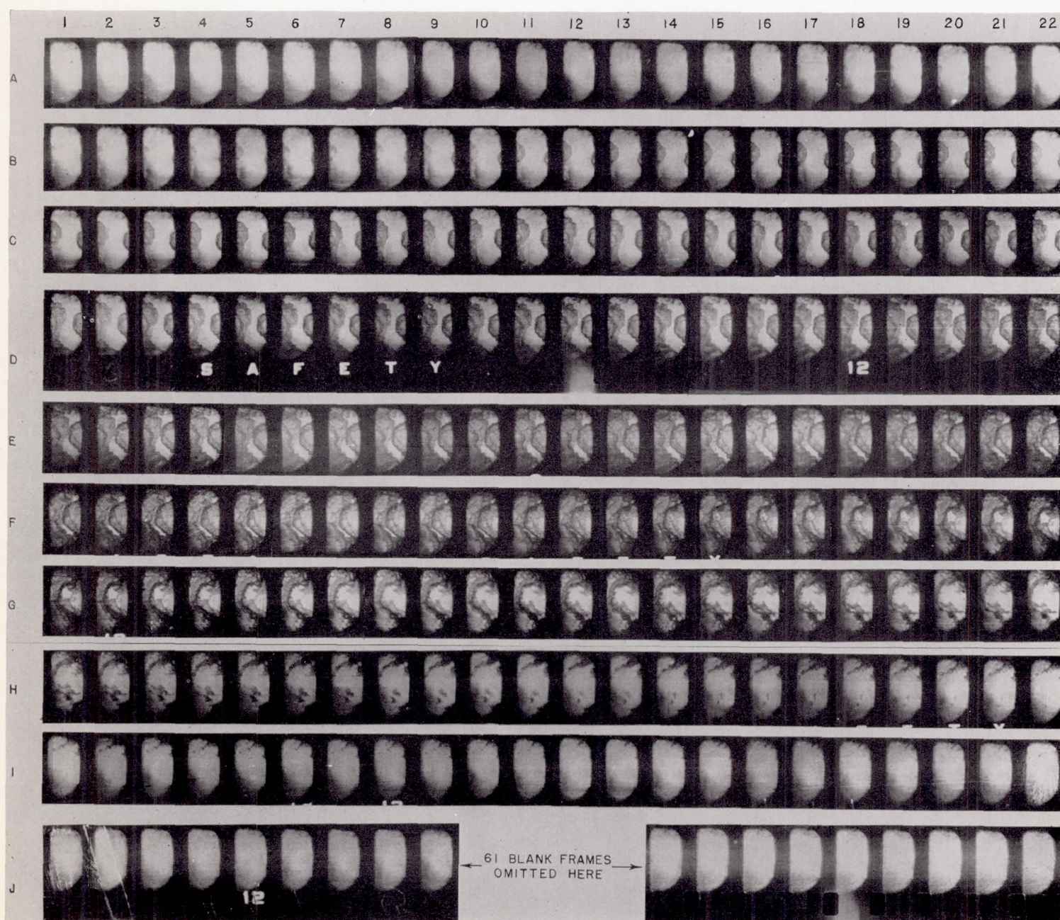
FIGURE 15.—High-speed motion pictures of an explosion in a spark-ignition engine without knock. Fuel, S-1; four spark plugs; spark advance, left-hand plug, 29^\circ , other three plugs, 22^\circ .
