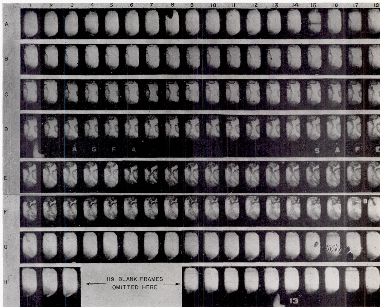
FIGURE 7.—High-speed motion pictures of an explosion in a spark-ignition engine with violent knock. Fuel, 50 percent S-1 with 50 percent M-2; four spark plugs; spark advance, left-hand plug, 29^\circ , other three plugs, 22^\circ ; B, blurring caused by knock.
