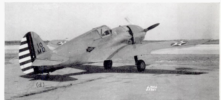
(a) Side view. (b) Three-quarter front view. (c) Close-up view. (d) Three-quarter rear view showing modified cowling flaps.
