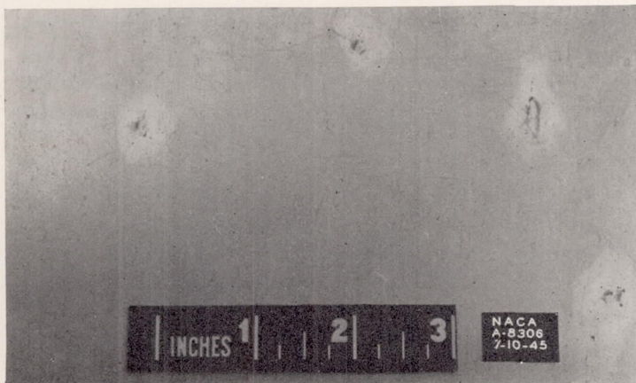
FIGURE 43.—Area of baffle plate shown in figure 42 after cleaning with acetone.
