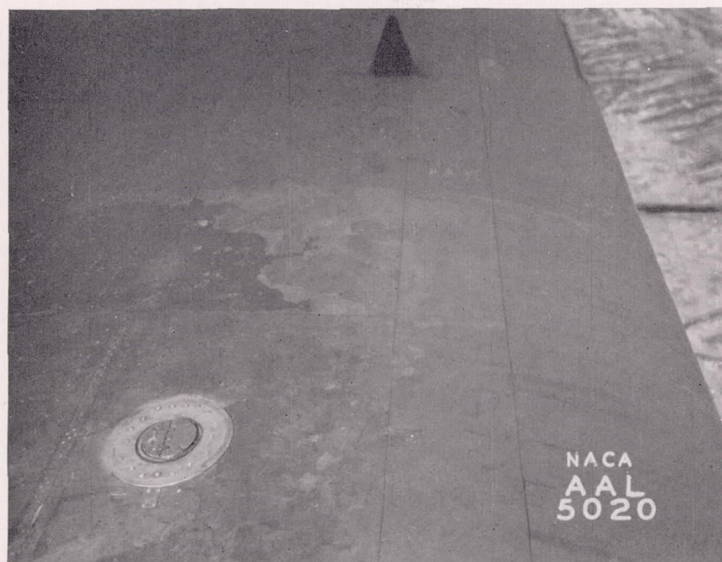
FIGURE 28.—Ice removed by engine warm-up and take-off in simulated icing tests.
