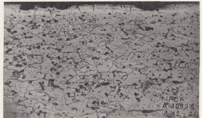
FIGURE 44.—Cross section of baffle-plate cladding and core beneath the synthetic rubber particle at section A-A, figure 42. Magnification, 200X; Keller's etch. Pitting is severe but has not penetrated the cladding.
