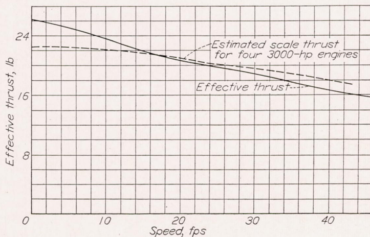
FIGURE 6.—Variation of effective thrust with speed. Model 180; trim, 0°; \delta\tau=30^\circ ; \delta\theta=0^\circ .
