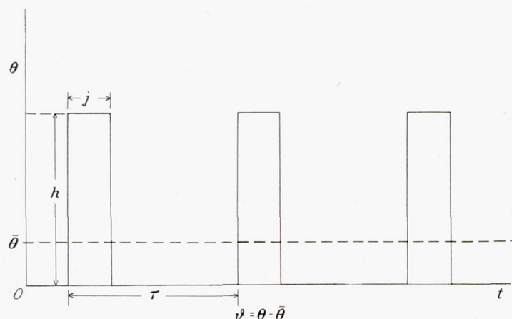
FIGURE 35.—Simulation of temperature signal close behind local heat source.
