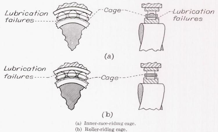
FIGURE 1.—Location of lubrication failures at cage-locating surfaces of rolling-contact bearings.
