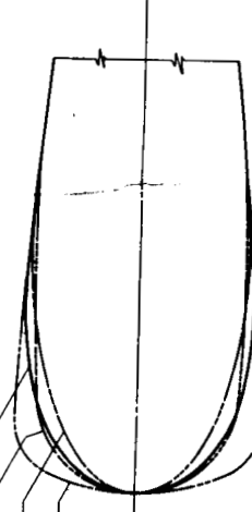
FIGURE 3b: MODEL SBD-1: REPRESENTATIVE HORIZONTAL SURFACE AIRFOIL SECTION WITH FINAL ELEVATOR BALANCE NOSE SHAPE AIRFOIL: MODIFIED N-69 WITH 12% CHORD EXTENSION AND STRAIGHT SIDED AFTERBODY, THICKNESS VARIABLE FROM 10.9% TO 7.5% ALONG SPAN ELEVATOR TRAVEL: THEORETICAL LIMIT FOR UNPORTING: \pm 24^\circ DESIGN STOPS AT 30^\circ UP, 20^\circ DOWN SECTION TAKEN AT REFERENCE STATION 46: CHORD = 50.83 INCHES
