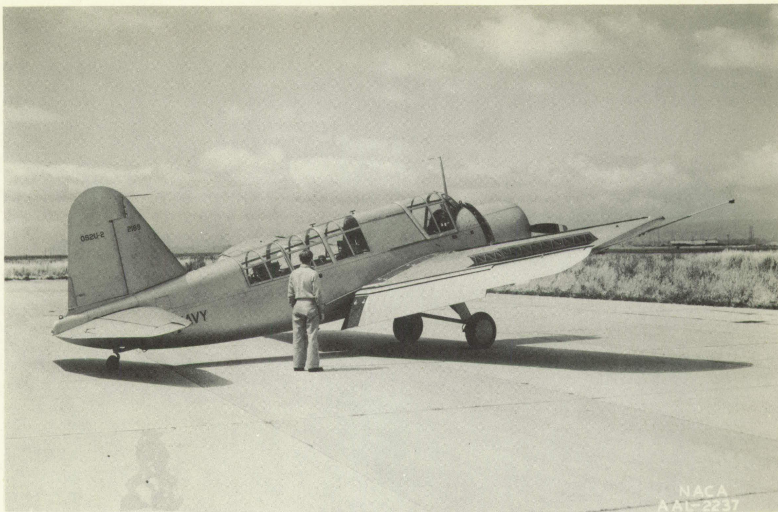
Figure 2.- Three-quarter rear view of the test airplane as instrumented for flight showing deflected flap, drooped aileron, deflected spoiler, and open slot.
