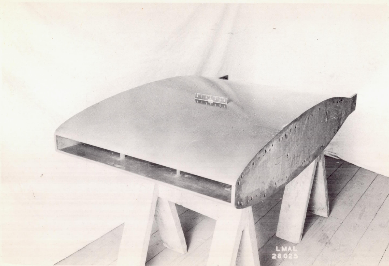
Figure 2.- View showing typical 60-inch-chord nose-opening model.
