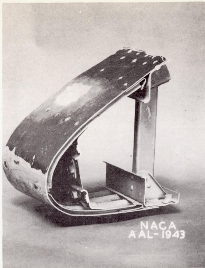
Figure 4.- Two views of the outer-panel wing leading edge anti-icing system of the Ju 88 airplane.
