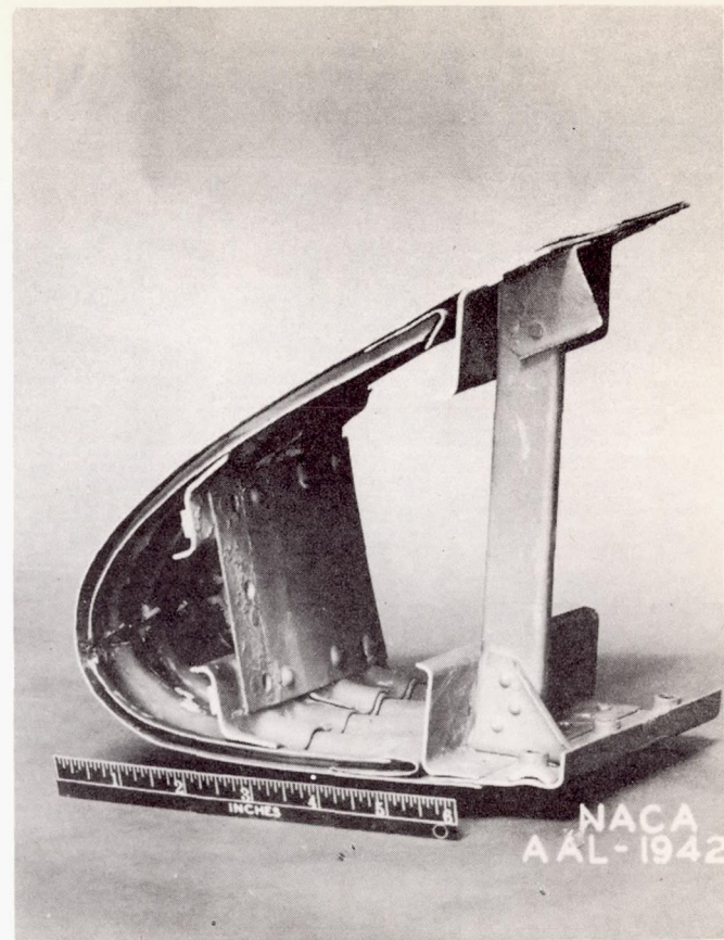
Figure 4.- Two views of the outer-panel wing leading edge anti-icing system of the Ju 88 airplane.
