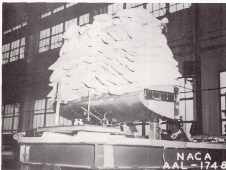
Figure 6.- The model heated leading edge being statically loaded. High angle of attack, load factor 6. Applied load 212 pounds per square foot.
