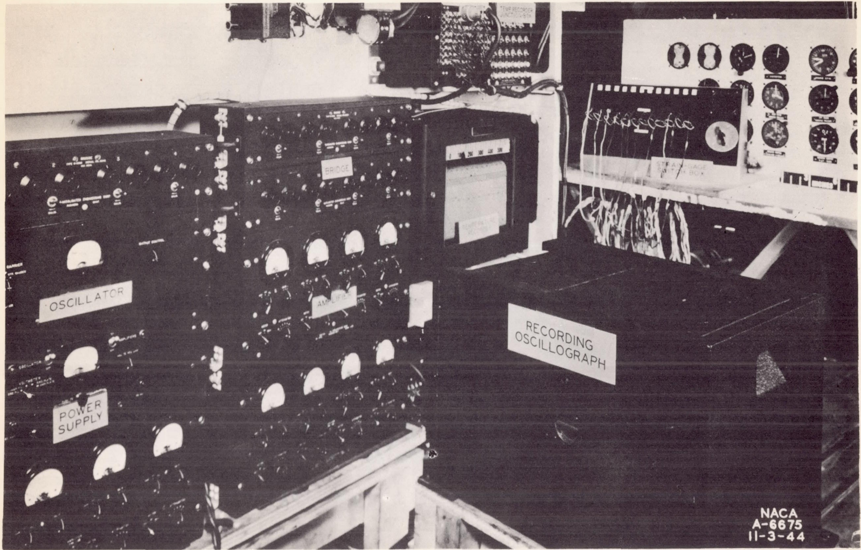
Figure 8.- Installation of instrumentation in airplane cabin for the wing thermal-stress investigation, C-46 airplane.
