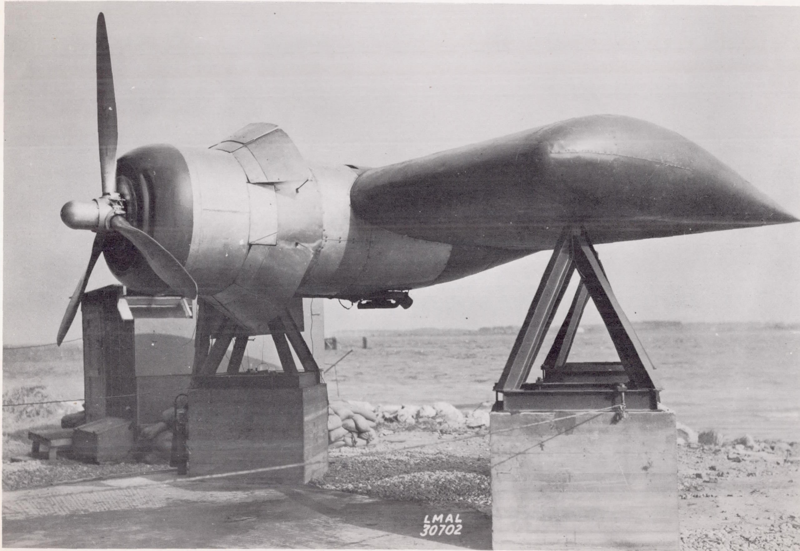
Figure 4.- Ground test setup of Pratt & Whitney R-1830-43 engine in the Consolidated B-24D engine nacelle.
