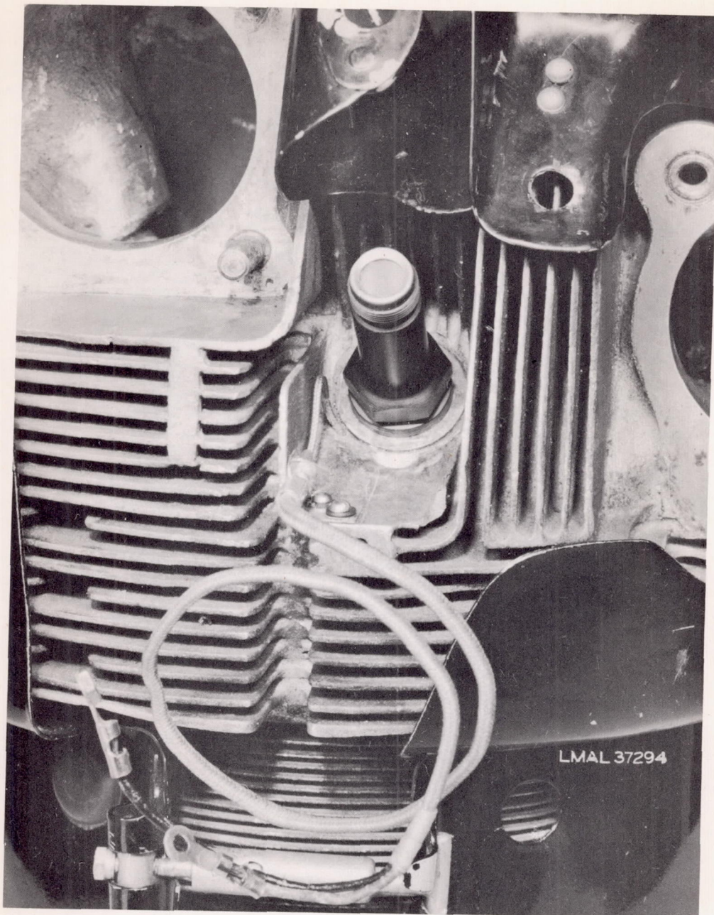
Figure 3.- Embedded thermocouple installed on front cylinder of R-2600 engine.
