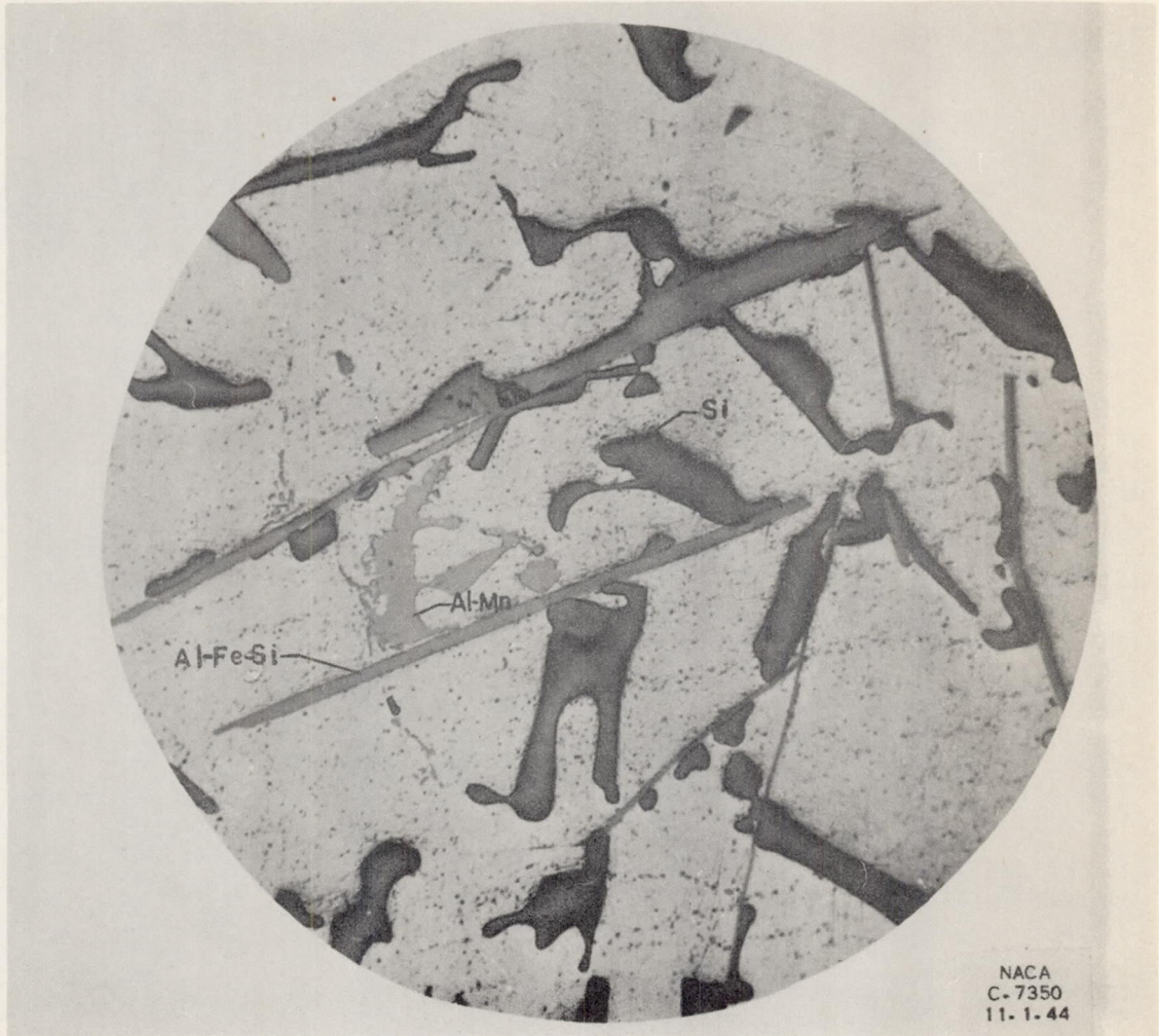
(a) From top of impeller 2-23. Etched in hydrofluoric acid.
