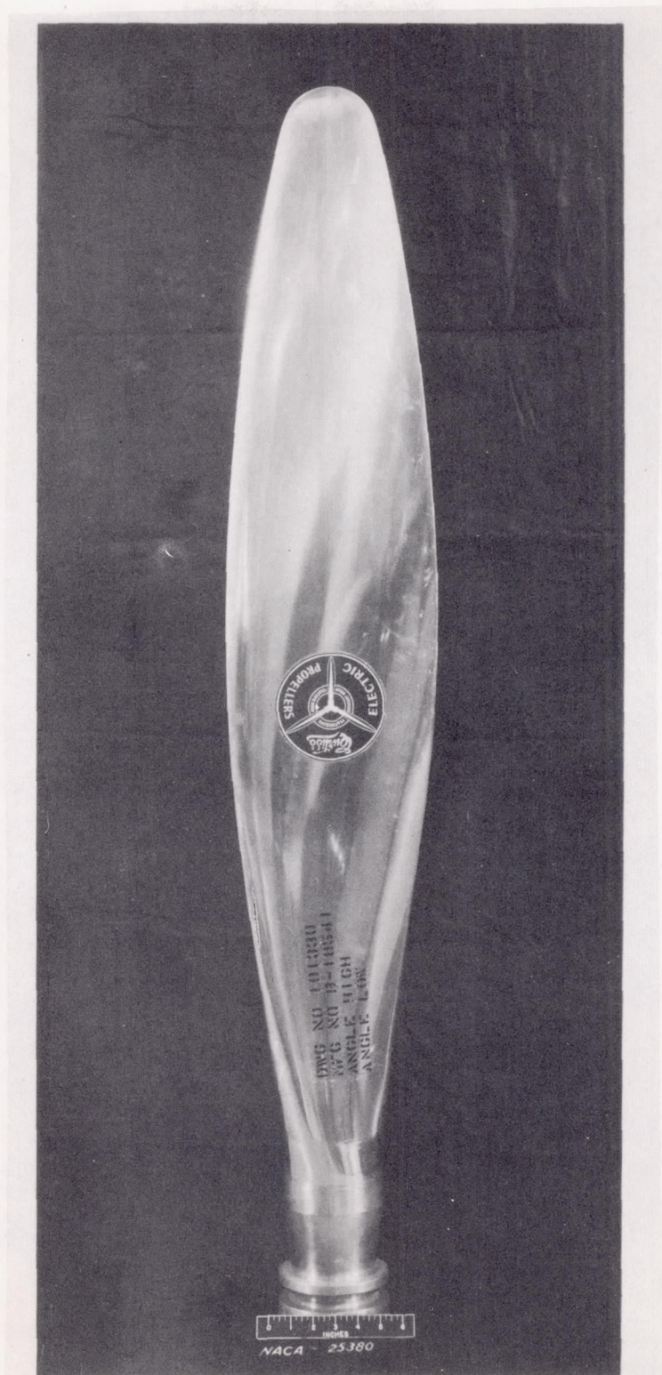
Figure 3.- Photograph showing plan form of all the propeller blades tested.
