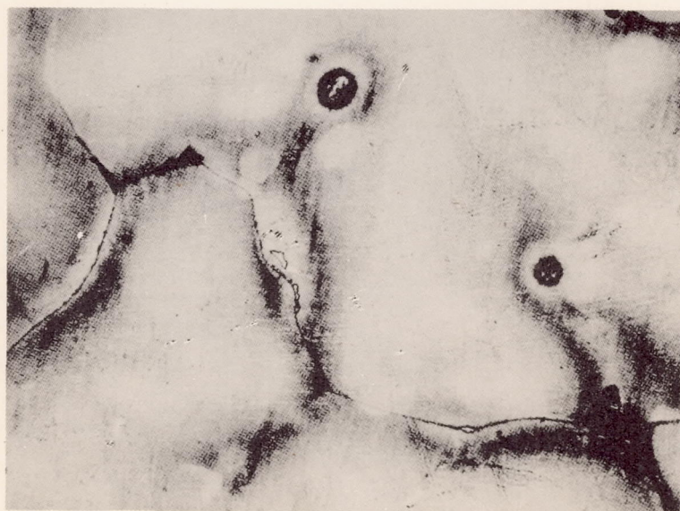
FIG. 8d Same as Fig. 8c. Etched with 10% NaOH solution in water. The CuAl 2 rosettes are light and the \alpha Al-Fe-Si constituent is black.
