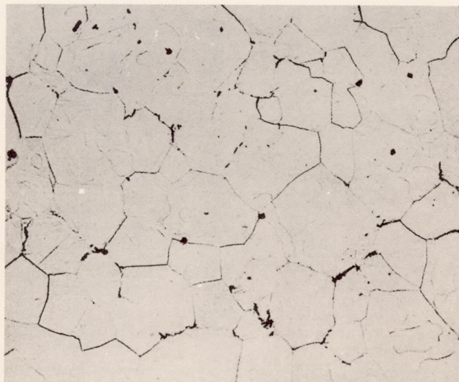
FIG. 8b Photomicrograph at X100 of an alloy containing 0.34% Cu, 0.17% Fe, 0.08% Si, 7.02% Zn, 0.18% Ti, 0.33% Mg and 0.26% Cr. Keller's etch.
