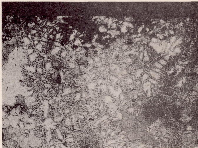
Figure 10.- Interdendritic attack in extruded 24S-T aluminum alloy, specimen 36989-1. Magnification, 100 diameters.
