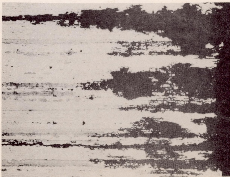
Figure 11.- Interfragmentary attack in extruded 24S-T aluminum alloy, specimen 26076. Magnification, 100 diameters.
