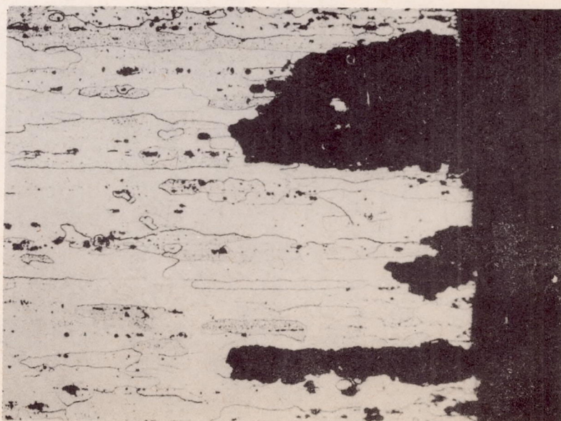
Figure 2.- Pitting type of edge at- tack in 24S-T alu- minum-alloy tubing, specimen 45974. Magnification, 100 diameters.
