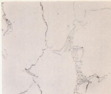
100X 1000X (a) Original microstructure - As cast. Electrolytic Sodium Cyanide etch - Vickers hardness 290.
