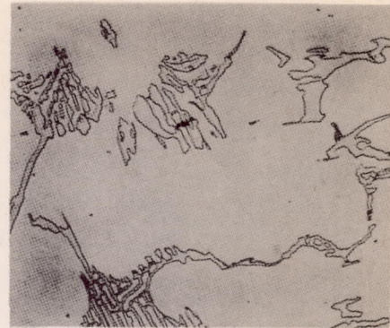
(a) 100X Original microstructure - As cast. Electrolytic Sodium Cyanide etch - Vickers hardness 286.
