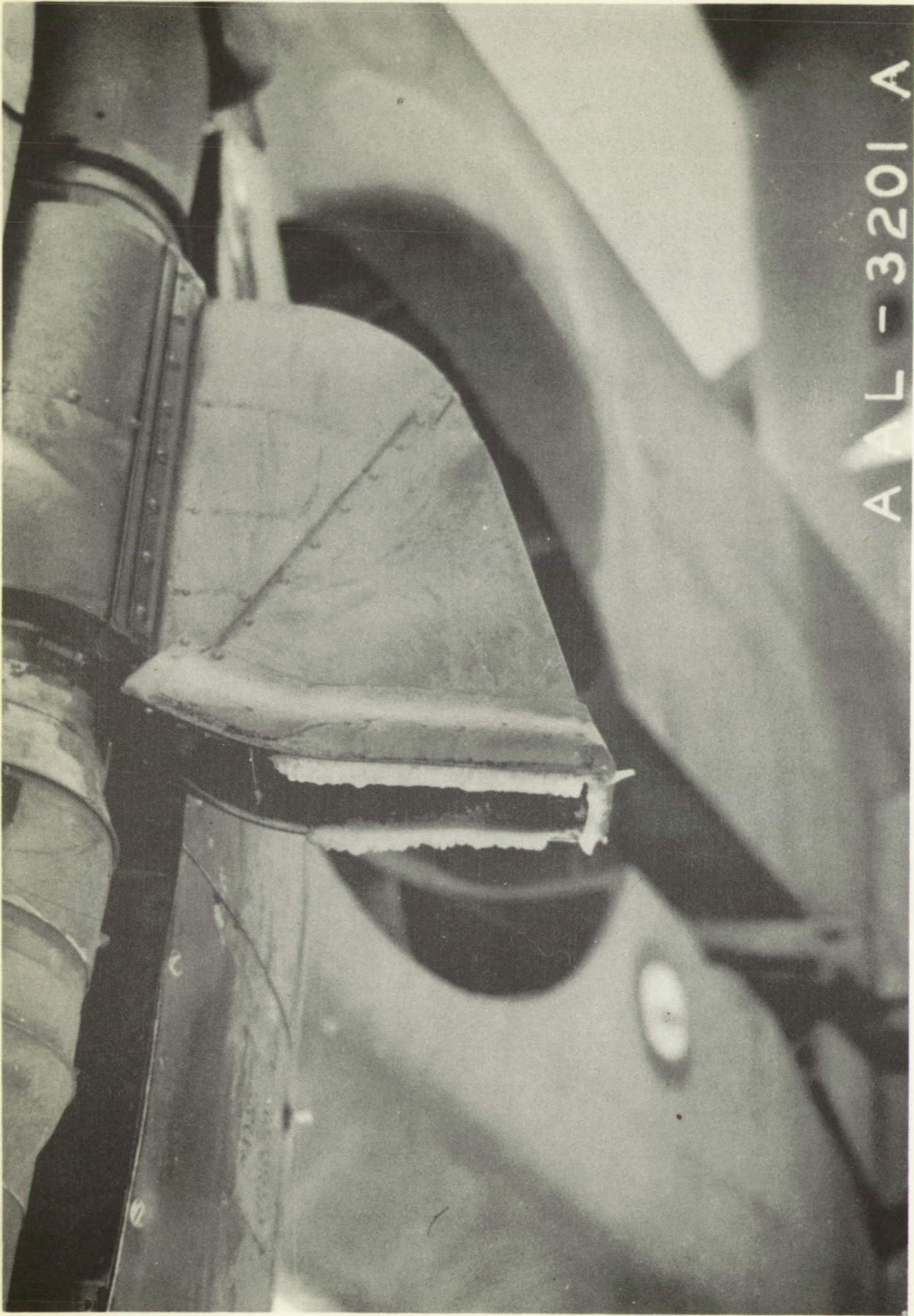
Figure 23.- Rime-ice formations on the heated lips of an air-intake scoop. Test 13.
