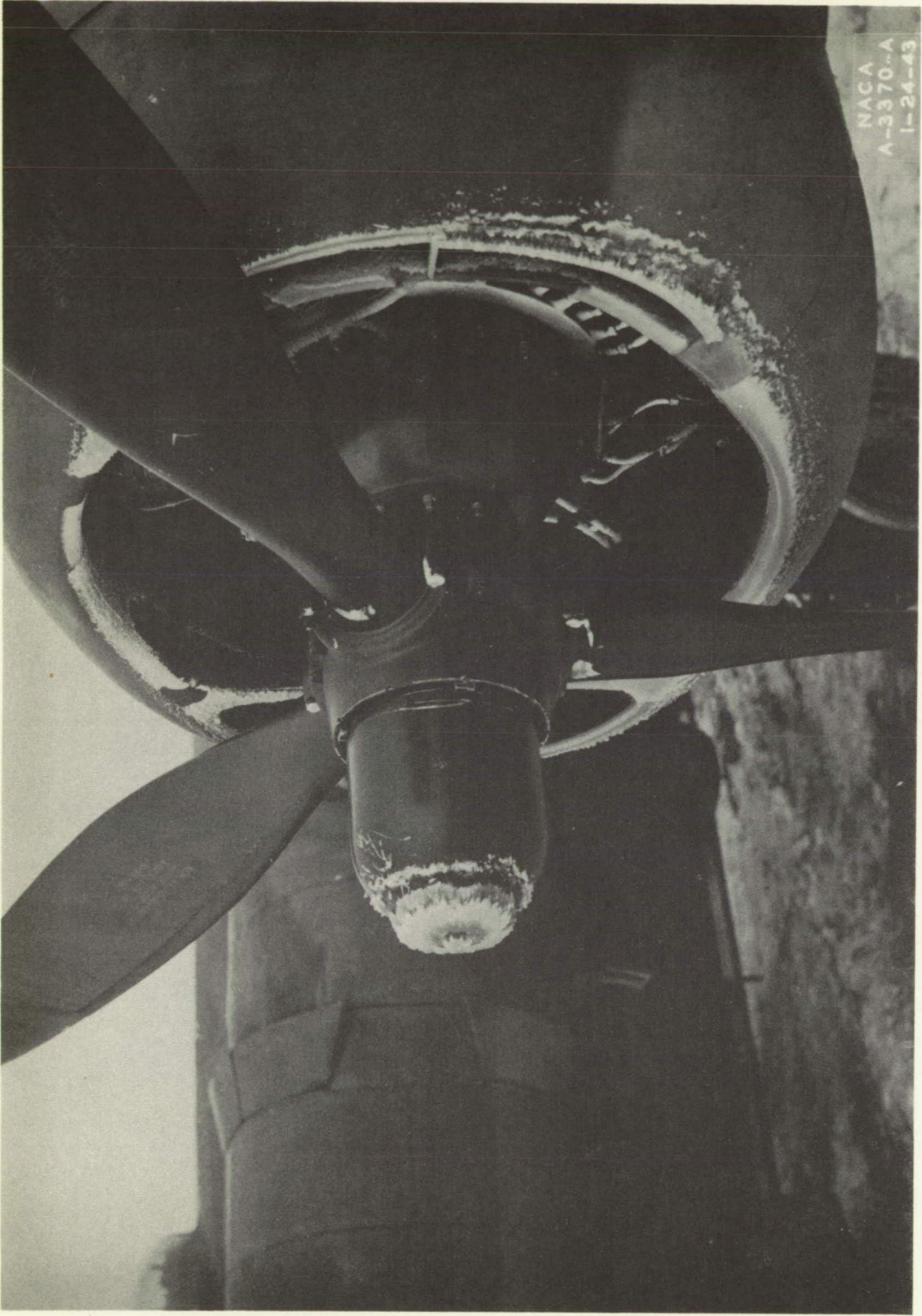
Figure 24. - Rime-ice formations on the propeller spinner and engine-cowl leading edges. Test 7 and 8.
