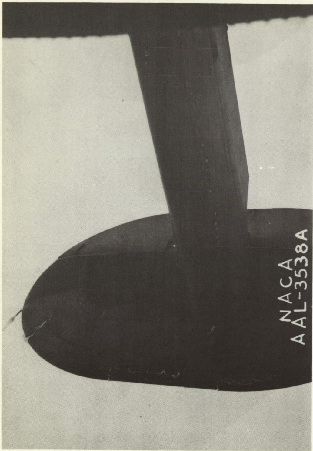
Figure 14.- Right horizontal stabilizer and vertical fin during flight in glaze icing conditions. Test 9.
